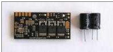
Important note: polarity - the white, thick-minus mark of capacitors must be on the board margins
