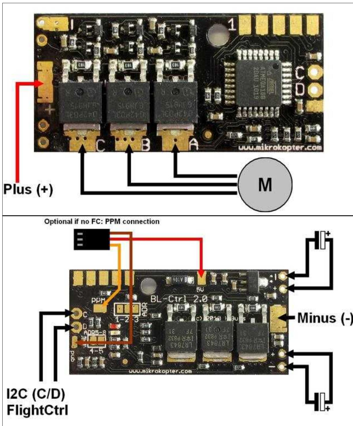
**INFO:** Normally you connect the BL-Ctrl on the "I2C-Bus" of the [FlightCtrl](#) and set the needed address with a solder-bridge on the BL. But if you want to connect the BL-Ctrl with an PPM-cable (see second picture: PPM connection), an addressing with a solder-bridge is not necessary.
