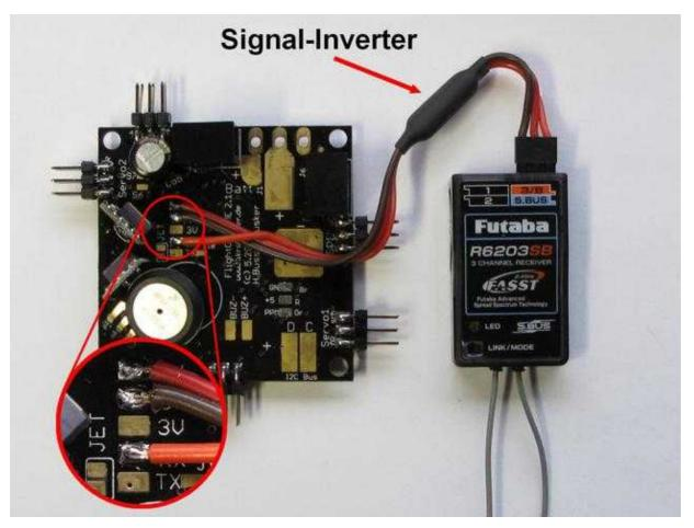
Since this version receiver from Futaba with the S.Bus will be also supported. Connected are those by a Signal-Inverter to the FlightCtrl.
