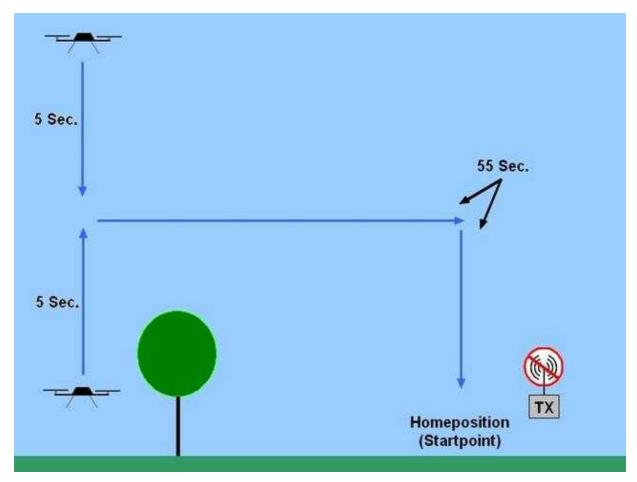
During a loss of a signal it is now possible to activate automatically a "FailSafe"-Function throughout the Kopter.
