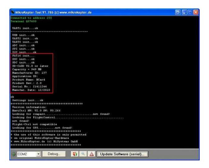
If you want to read or change the data on the Micro SD-card, it must be removed from the <u>NaviCtrl</u> and plugged into an appropriate card slot on the PC.
