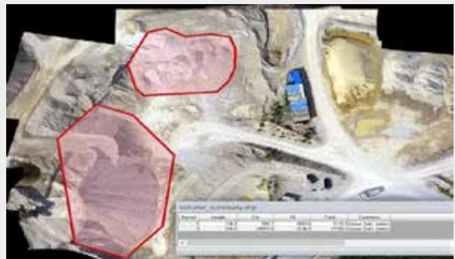
The created Point Clouds with the 6sGEO-II and an appropriate software reveals the volume of the needed area.
